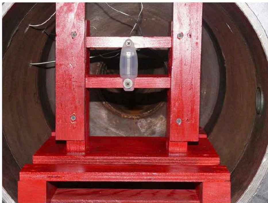
Figure B-3. E/T Light ® Model No. v6.8 IR, Installed in Test Chamber, Prior to Test.
