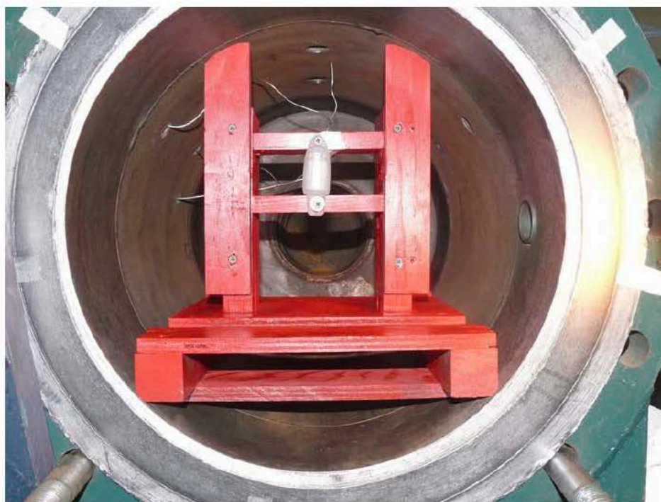
Figure B-2. E/T Light ® Model No. v6.8 A, Installed in Test Chamber, Prior to Test.
